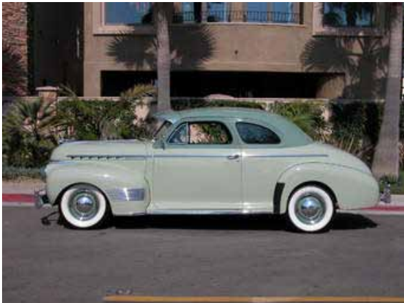
1941 Chevrolet two-door coupe, with 85 HP, 6-cylinder engine with 216.5 cubic inch displacement.
